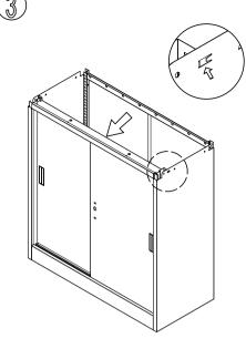
Fix the door frame onto both of the side plates.
